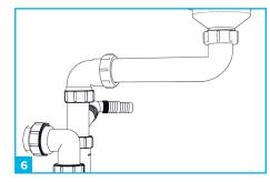
Now Insert the pipe section into the 90° bend and tighten all nuts for a watertight seal.
