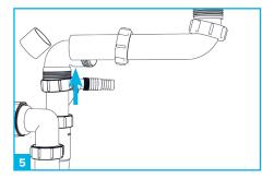
Now you need to cut the pipe section to suit. Connect the pipe section of the kit to the bottom of the waste. Mark and cut the pipe section just short of where the 90° bend narrows.
