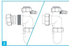
Attach the trap to the outlet pipe, by removing the nut, slip ring and conical washer, placing them over the outlet pipe and then screwing onto the trap outlet
