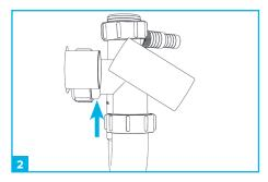
In order to save as much space as possible, cut the outlet pipe as short as possible. To do this, line up your trap with it's outlet against the back of the unit and cut the pipe where the trap outlet narrows. Smooth the cut edge with a piece of sand paper or file.
