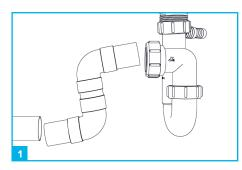
Start by disconnecting your trap and removing any surplus pipe work between it and the outlet.
