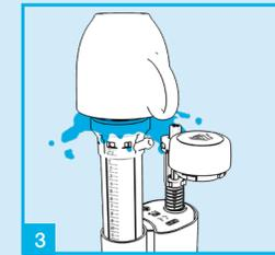
Turn the water supply on and off to clear any debris. Hold a cup over the top to prevent any splashing.
