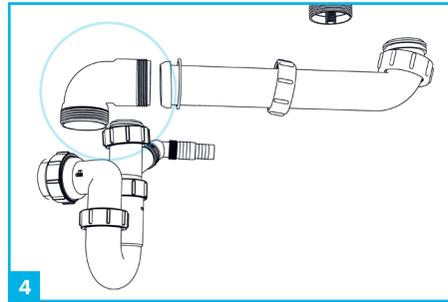
4 Now the trap is ready for the space saver kit. Take the 90° bend and attach loosely to the top of your trap.
