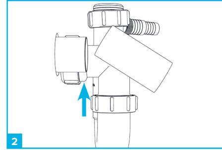
2 In order to save as much space as possible, cut the outlet pipe as short as possible. To do this, line up your trap with its outlet against the back of the unit and cut the pipe where the trap outlet narrows. Smooth the cut edge with a piece of sand paper or file.
