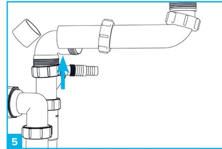
5 Now you need to cut the pipe section to suit. Connect the pipe section of the kit to the bottom of the waste. Mark and cut the pipe section just short of where the 90° bend narrows.
