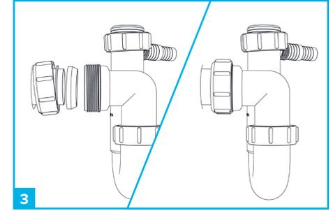
3 Attach the trap to the outlet pipe, by removing the nut, slip ring and conical washer, placing them over the outlet pipe and then screwing onto the trap outlet thread.
