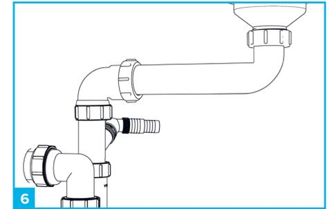
6 Now Insert the pipe section into the 90° bend and tighten all nuts for a watertight seal.
