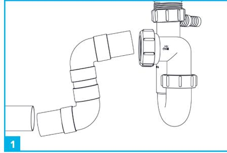
1 Start by disconnecting your trap and removing any surplus pipe work between it and the outlet.
